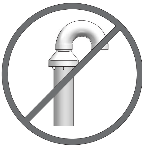
Figure 5-5 Do Not Install U-Bend to Rain Cap
